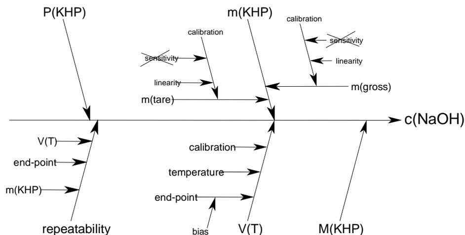
Figure A2.8: Cause and effect diagram (Repeatabilities combined)
